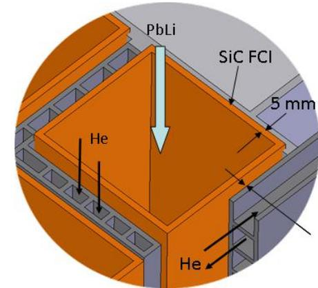
The electromagnetic *Lorentz force* is orders of magnitude higher than viscous or inertial forces, strongly affecting LM flows in the blanket
