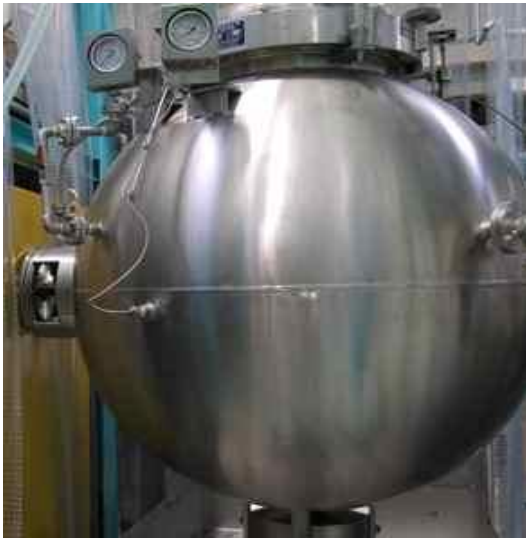
Pressure cooker (Max temp. 180°C, Max press. 1.0 Mpa)
