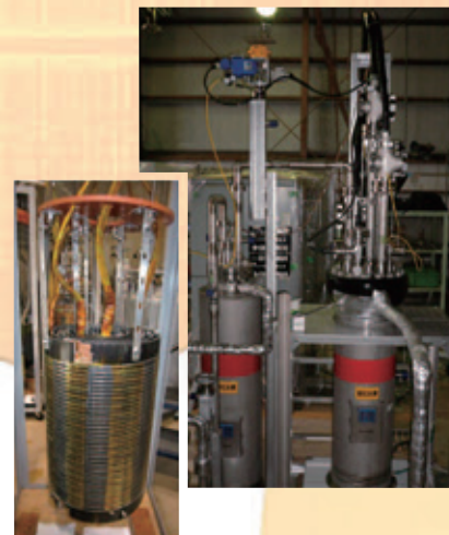
Experimental Setup for Liquid Hydrogen cooled Superconducting Energy Devices (right) and HTC Superconducting Fault Current Limiter (left)
