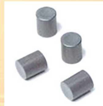
Uranium dioxide pellets for nuclear fuels in light water reactors
