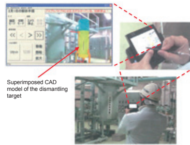
Dismantling planning support system based on augmented reality technology
