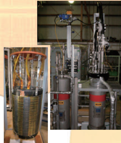
Experimental Setup for Liquid Hydrogen cooled Superconducting Energy Devices (right) and HTC Superconducting Fault Current Limiter (left)
