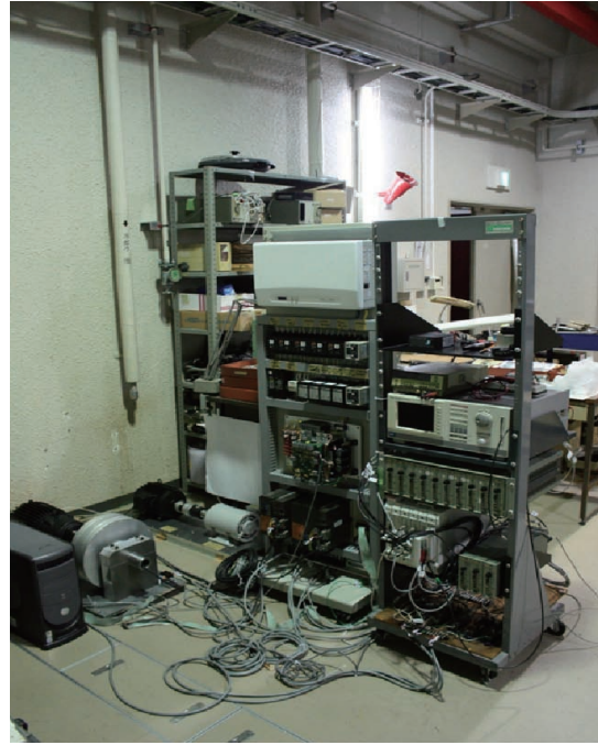
Figure 2. Photo of laboratory scale prototype model of hybrid offshore-wind and tidal turbine system with flywheel.
