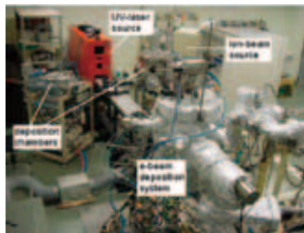
Electron-beam deposition and pulsed-laser deposition systems for fabrication of high-quality thin films
