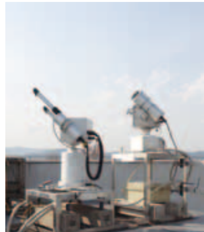
System for assessment of the radiative effects of atmospheric aerosols
