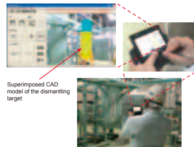
Dismantling planning support system based on augmented reality technology
