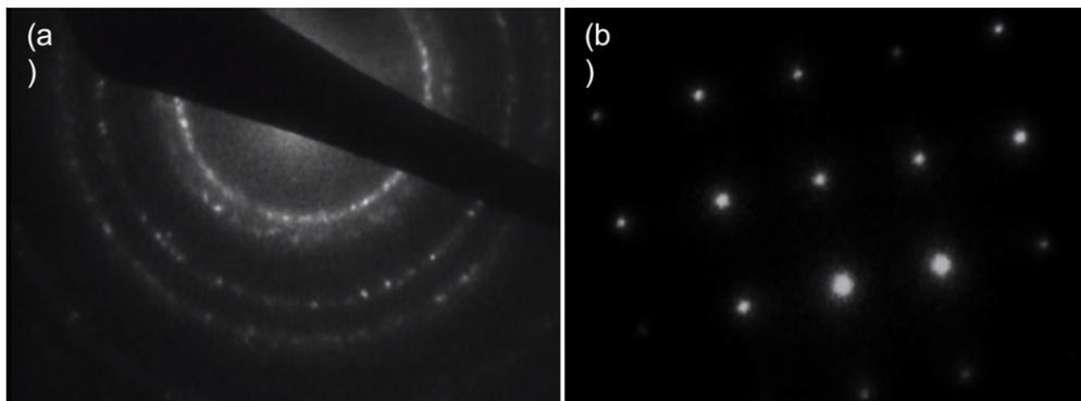
Figure 2 (a) Electron diffraction patterns of (a) NaCl polycrystal (Fcc) and (b) NaCl single crystal ([001] zone axis).
