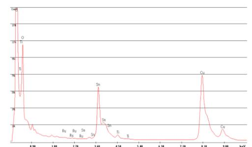
Figure 3 EDS spectrum of Ru-Sn catalyst grafted on TiO<sub>2</sub>.
