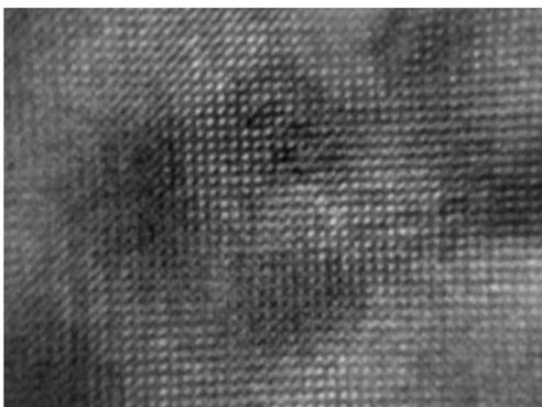
Figure 1 TEM image of Au thin layer. Accelerating voltage: 200kV. Magnification: ×1,000,000.
