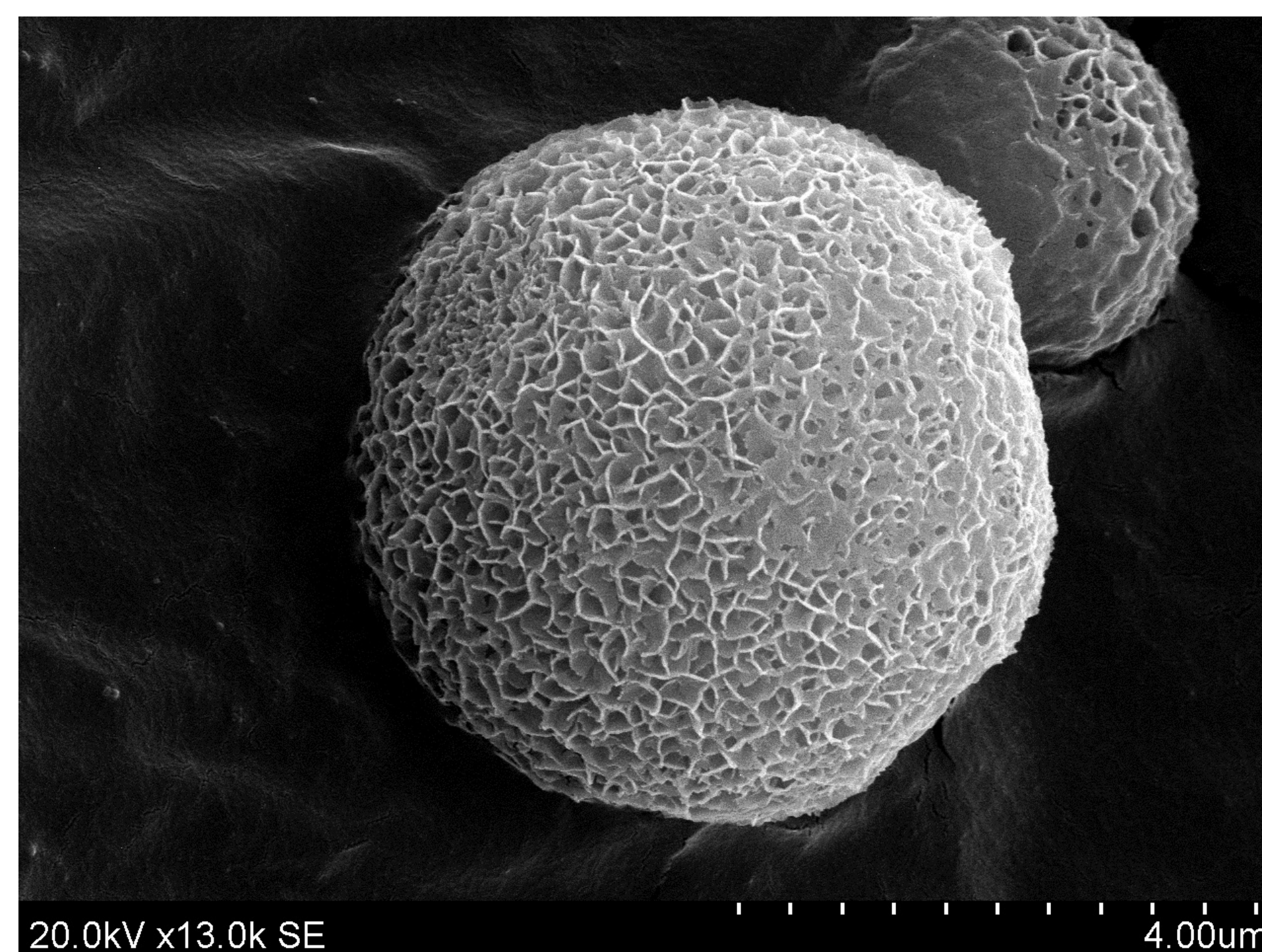
Figure 2. FE-SEM micrograph of microcapsules consisted of flake-like crystallites of hydroxyapatite formed in simulated body environment.
